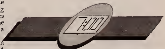
The display numbers in digital watches, as well as calculators, are made up of polymeric liquid crystals.
